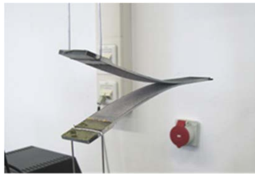
Figure 3-1: DCB sample while crack propagation
