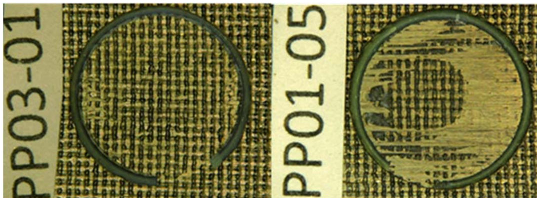
Figure 5-4: Fracture modes (left: low plasma treatment; right: amin blushing of adhesive)
